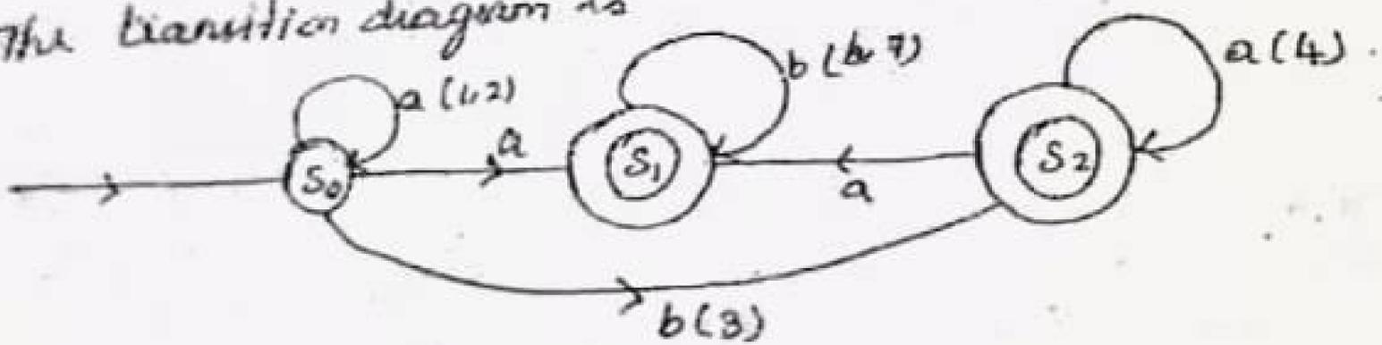
The path  $(S_0, S_0, S_0, S_2, S_2, S_1, S_1, S_1)$  represents a string  $\alpha = aabaabb$ . Since the final states  $S_1$  are accepting states, the string  $\alpha$  is accepted by the above NFA.
